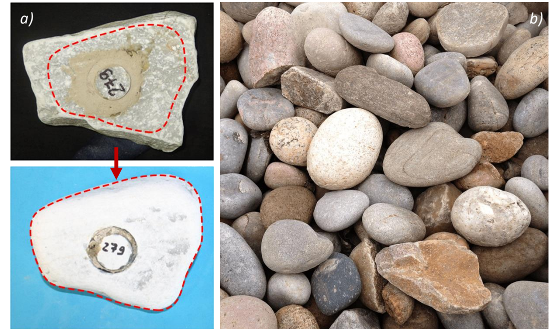
a) Particle rounding from abrasion in bed-load transport* b) Beach pebbles in various states of wear
