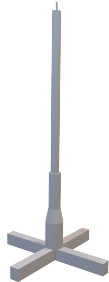
A tension-leg platform wind turbine
