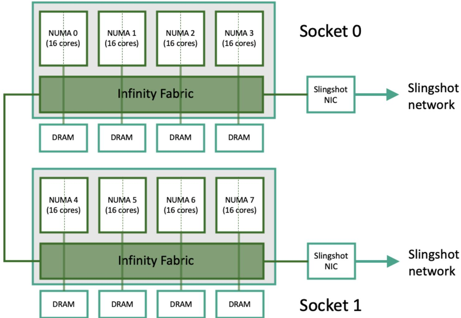
Each 16-core NUMA region is made up of 2 8-core compute complex dies.
