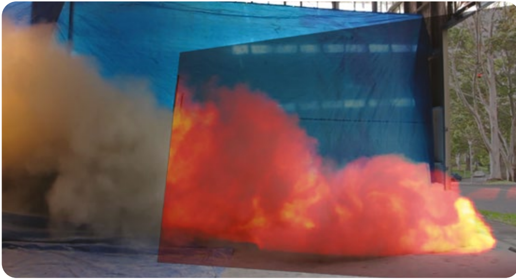
Figure 1: Side view of the PELE experiment, where an infrared image is overlaid on the visible image. The flow is 2m high on the left side of the picture.
