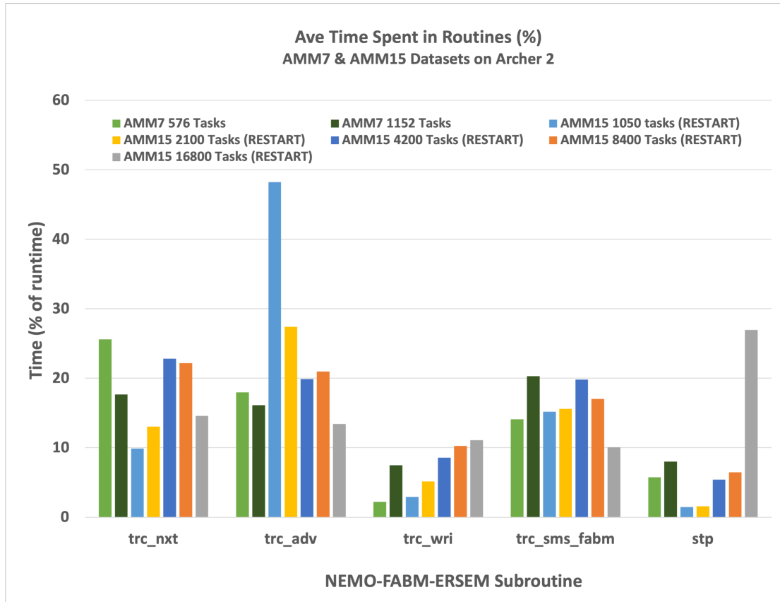
Figure 4 Timing Breakdown by Routine (Average time (%) across MPI processors)
