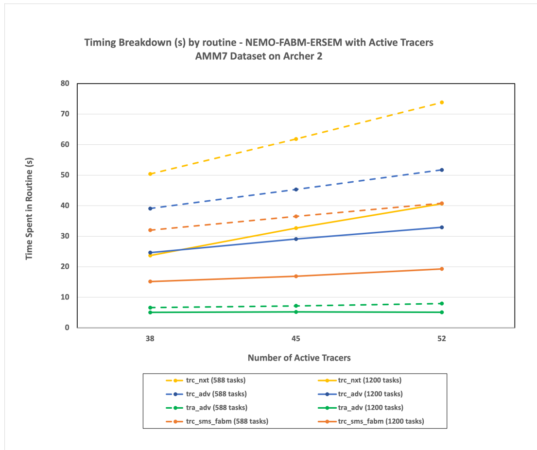
Figure 7 Timing breakdown (secs) by subroutine for 588 & 1200 MPI task NEMO-FABM-ERSEM runs involving varying numbers of active tracers (AMM7 Dataset)
