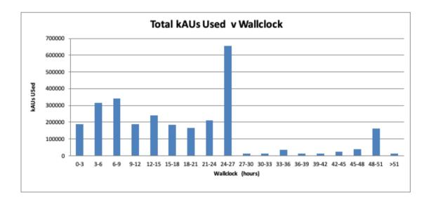
From the first graph, it would appear that the system is dominated by short jobs. However, the second graph shows that actual usage of the system is more spread and dominated by jobs of around 24 hours with a second peak for jobs around 48 hours.
