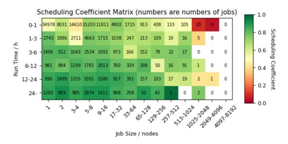
The usage heatmap below provides an overview of the usage on ARCHER over the quarter for different job sizes/lengths. The colour in the heatmap indicates the number of kAUs expended for each class, and the number in the box is the number of jobs of that class.
