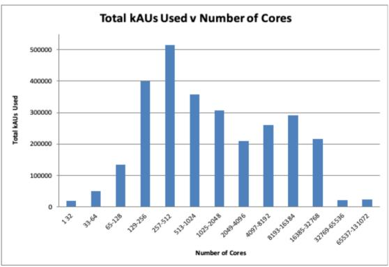
The first graph shows that, in terms of numbers, there are a significant number of jobs using no more than 512 cores. However, the second graph reveals that most of the kAUs were spent on jobs between 129 cores and 16384 cores. The number of kAUs used is closely related to money and shows better how the investment in the system is utilised.
